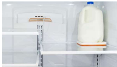
Slika 1: ChillHub - modul za tehtanje mleka ( https://www.cnbc.com/2015/01/05/this-smart-refrigerator-makes-your-fridge-look-dumb.html )
